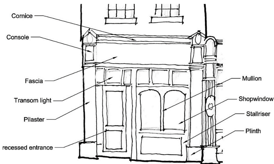
Figure 53 A diagram of a typical shopfront
