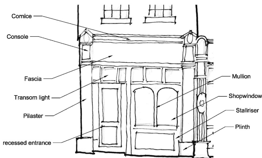
Figure 50 A diagram of a typical shopfront
