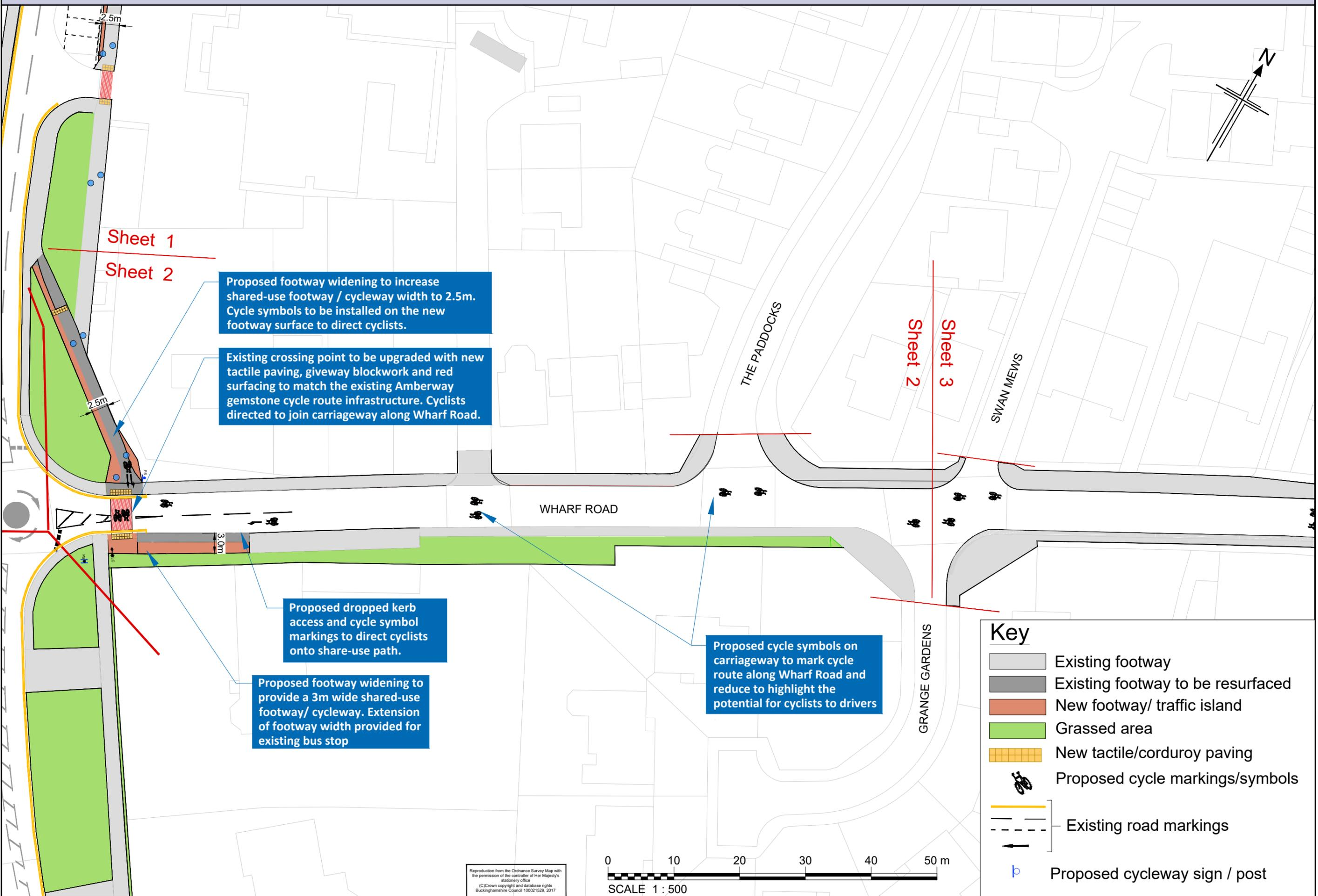
Proposed footway widening to increase shared-use footway / cycleway width to 2.5m. Cycle symbols to be installed on the new footway surface to direct cyclists.
