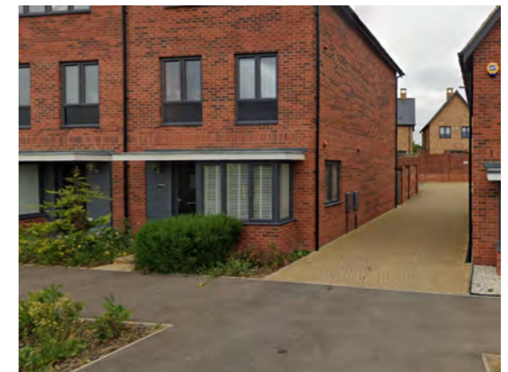
Parking is found to the rear of properties in courtyards. There can be problems with security unless there is sufficient overlooking.
