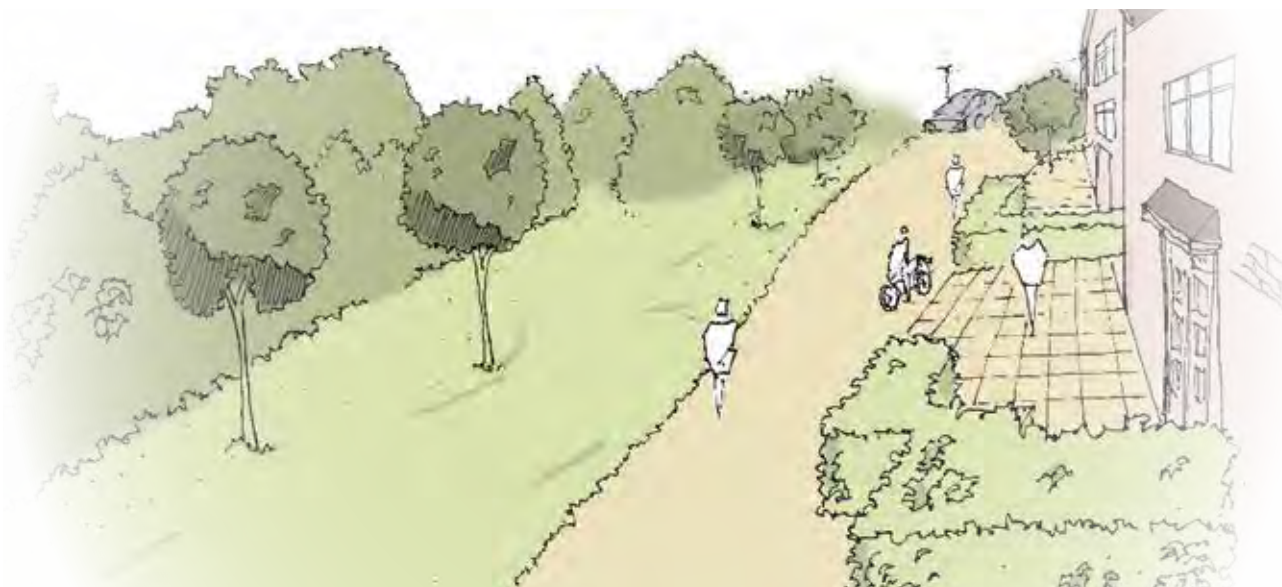
Figure 67: Sketch to illustrate design guidelines on how new development can treat the rural edges by facing onto them improving natural surveillance and allowing for open views to the countryside.
