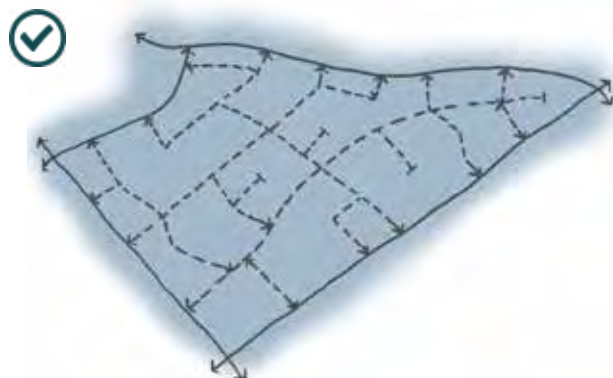
Figure 52: A connected layout, with some cul-de-sacs, balances sustainability and security aims in a walkable neighbourhood.
