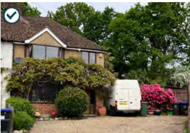
Figure 64: Positive example of on-plot parking laid with permeable gravel paving, Elizabeth Way.
