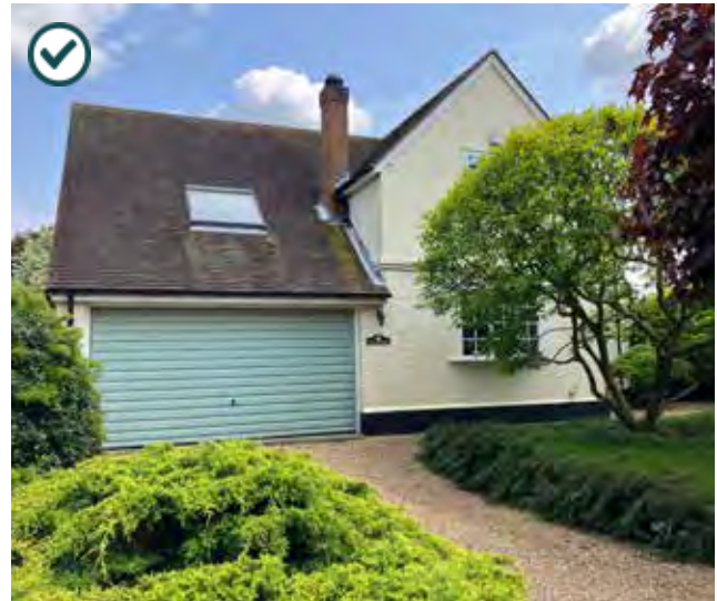
Figure 47: Positive example of on-plot parking with garage on the side of the building, aligned with the principle building line, with permeable driveway ground surfacing.
