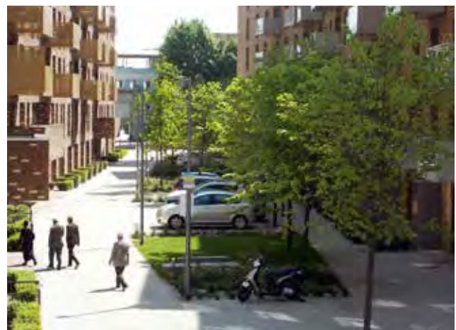
Figure 49: Example of on-street parking with planting used to break up parking bays, St Andrews, Bromley-by-Bow.
