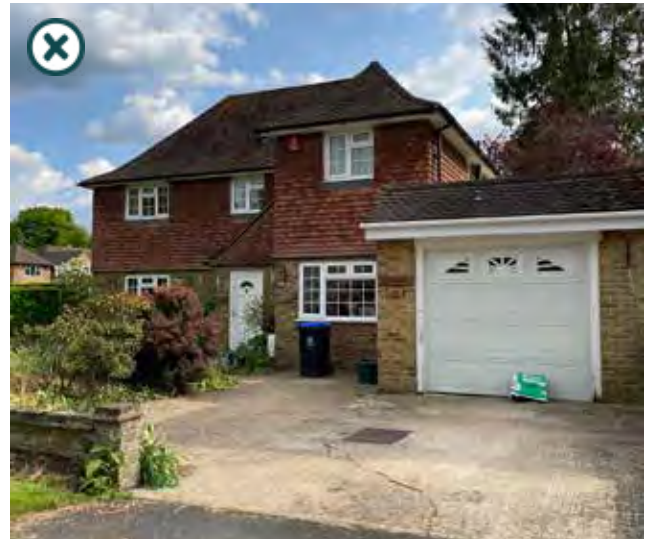
Figure 48: Negative example of on-plot parking with attached garage at the side of the building, dominating the principle building line, with impermeable driveway ground surfacing.
