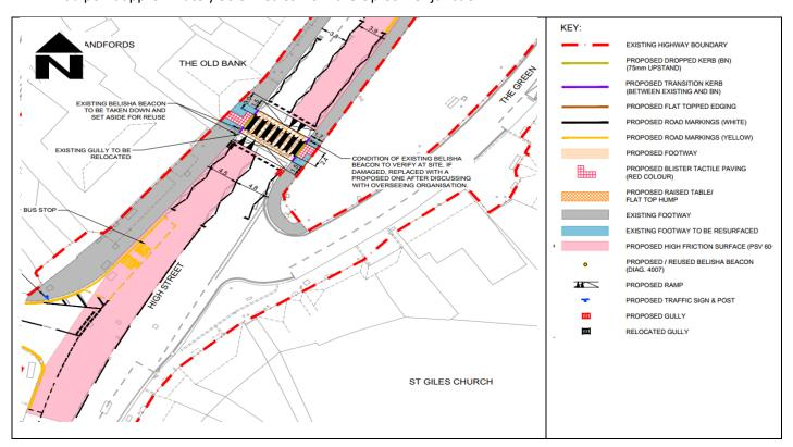
The Raised Table proposal is to improve the safety for pedestrians wishing to cross High Street using the new facilities, with drivers encouraged to approach at a reduced speed. The suburban and residential setting, and the proximity to commercial sites within the village centre, the scheme seeks to benefit local residents and shoppers, when crossing at this location.
